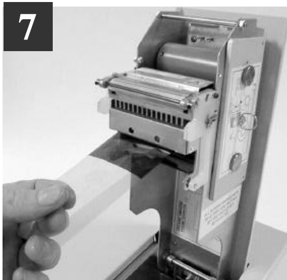
7 Pull about 6" of dye film off the roll of dye film, observing that it should be coming off the top of the roll, as per the label illustrations.
